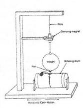
Different devices are used to measure intensity of earthquake one such is shown in figure. We can take some precautions when we are outside or when we are inside out home. Based on above extract answer the following questions;
