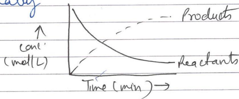
However, the rate of reaction is also found to decrease. This shows that the rate of reaction is directly related to the concentration of reactants. The effect of concentration on reaction rate was first studied by Arrhenius and Waage in 1867 in the form of law of mass action. For a general reaction  $aA + bB \rightarrow \text{Products}$
